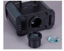
Unscrew and remove the focus lens. Using your thumb, gently push the lens outward until it "pops" out.
